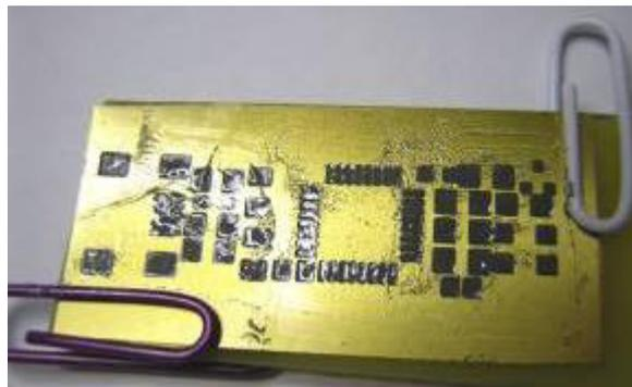
Take the mask off the circuit board. Try to remove it vertically so that solder nicely stays on the board.
