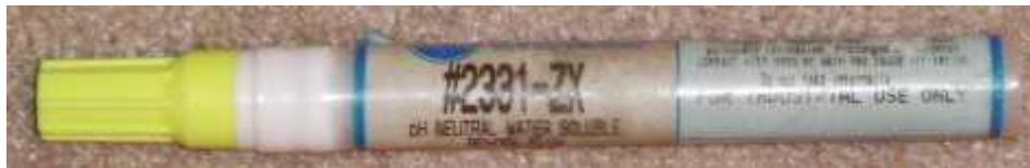
Some form of liquid flux will be necessary for getting the solder to flow well. I use a Kester 2331-ZX flux pen which is stocked by Digikey. The flux pen I have recommended contains water soluble flux which makes cleaning the board easier, but will corrode the board in not cleaned within a few hours of soldering. This flux is also conductive.
