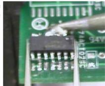
**Step 5** Suck the solder off the pads ready for the new part.
