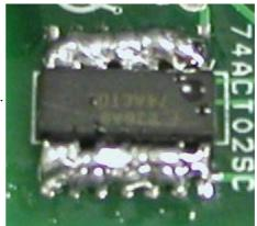
**Step 2** Heat one side and move the iron back and forth until the whole row of pins is melted. Insert the screwdriver under that side and pry up until the pins are off the PCB and out of the solder.
