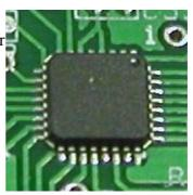
**Step 2** Spread a thin layer of solder paste across the PCB on the pad area for the BGA, MLF / MLA part. The thickness of the solder paste should be thin enough so that the PCB and pads should be semivisible. The amount is learned by trail and error and experience.
