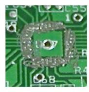
Step 3 Place the BGA, MLF / MLA part on the PCB and align. Use needle-nose pliers to hold the part in place while heating. Make sure the pliers are not bare metal or they will get too hot to handle when heating. Using the heat gun, apply
