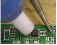
Finally inspect the pins to check if any solder is left between them. If there is, re-apply solder between the pins and re-suck. This method works because sucking only removes the solder between the pins and not the solder between the pad and pin.
