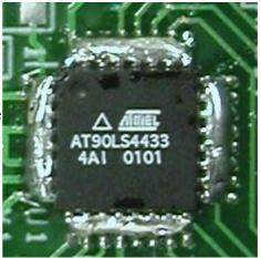
Step 4 Using the iron, (or a heated sucker) heat an end of a row until the solder is melted 2-3 pins in length from the end. Quickly remove the iron and using a solder sucker, suck the excess solder from between the pins. Heat the solder on the next 2-3 pins and do the same until the other end is reached. Do the same on the other three sides of the chip. Finally inspect the pins to check if any solder is left between them. If
