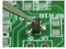
**Step 4** Now solder the other two pins, one-at-a-time. Use a chise tpye tip (1/32" wide). Contact the pin and pad at the same time with the conrner of the tip. Do not use the end of the tip or solder will flow from pin to pin.
