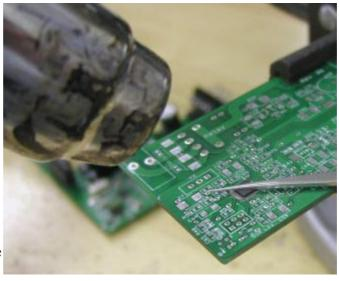
heat to the part by holding the heat gun 8cm (3") away from the board.
