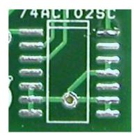
**Step 2** Grab the 14 pin SOP part with very fine tweezers. Bring the part overtop of the pads, sit the part on top of the pads. Heat the pad with solder and adjust the part so that it lines up with the pads. Besure the part is flat and aligned, then remove the heat.
